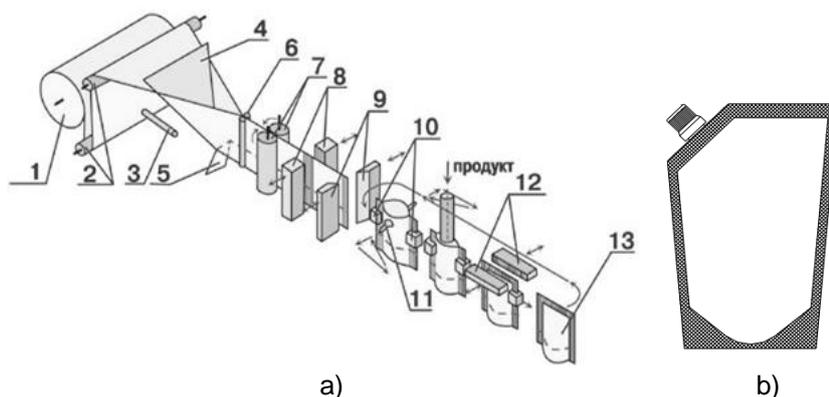
**Fig. 1.** Technological scheme of paste packing in packages "doypack" (a) and a package doypack with a cork (b), authors': 1-roll of film, 2- film unwrapping, 3-puncher, 4-pipe formation, 5-photosensor, 6,7- swaths, 8-longitudinal welding, 9-cutting, 10-package opening, 12- sealing of the package (in packages with the cork, between the cutting mechanism 9 and the mechanism of package opening
